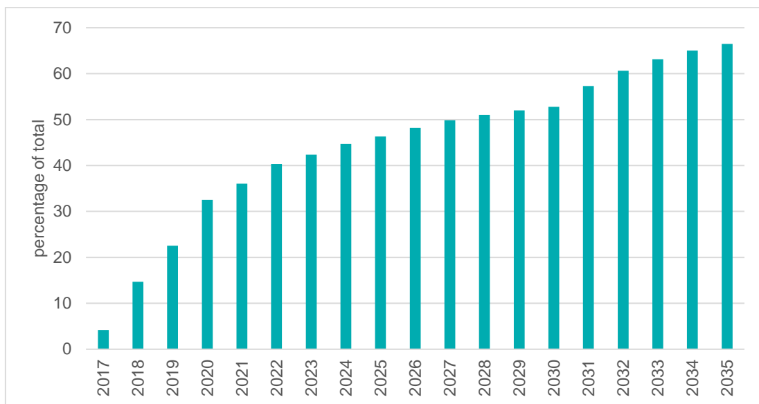
Figure 12: Import quota of electric cars for all new registrations of electric cars in the electromobility scenario
